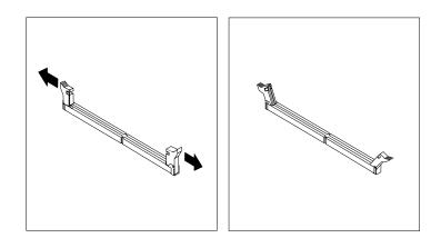
Figure 15. Opening the retaining clips
